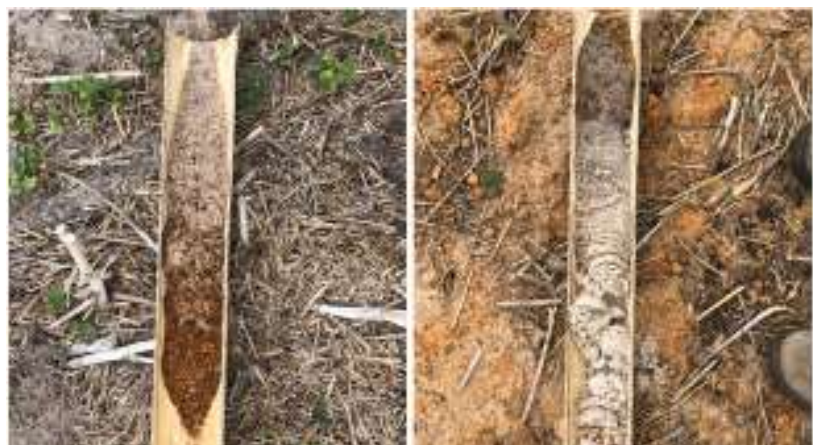
Figure 3: Soil types found at the site were either pale sand over gravel (left) or deep pale sand (right).
