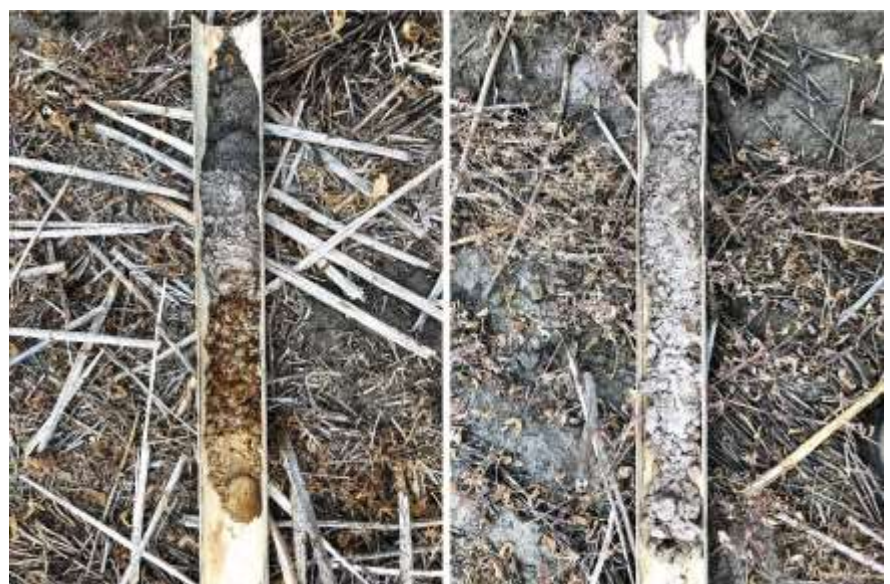
Figure 3: Soil types found at the site were either pale sand over gravel (left) or deep pale sand (right).
