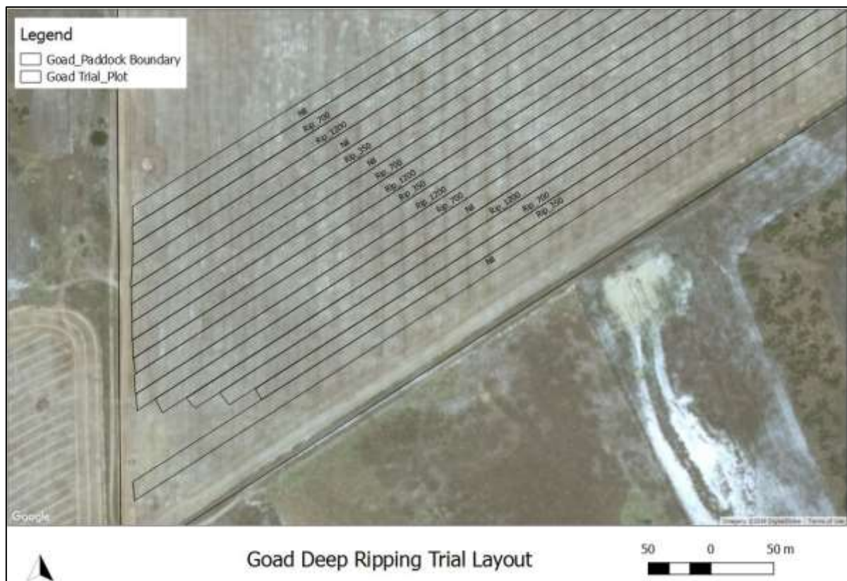
Figure 1: The deep ripping trial design on Josh and Tony Goad's farm near Kojaneerup was finalised in 2016. The trial consisted of three ripping treatments at 350mm, 700mm and 1200mm in 12 metre wide plots. Undisturbed 'Nil' plots allowed yield comparisons to be made in barley and canola crops in 2016 and 2017.
