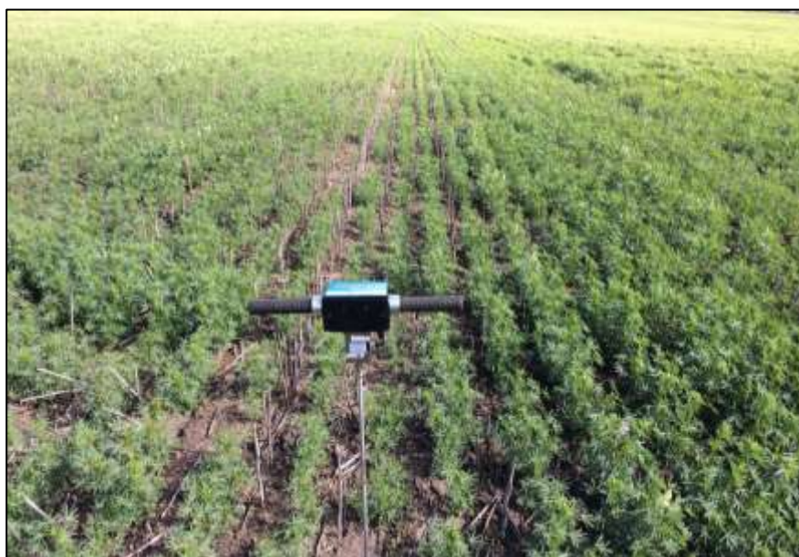
Figure 3: Rimick CP300 Cone Penetrometer used to record soil resistance across the trial site.
