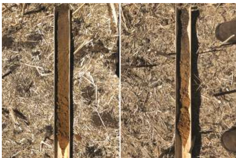
Figure 4: Soil types found at the site were either a loamy sandy over gravelly clay (left) or sandy gravel loam over gravel (right).
