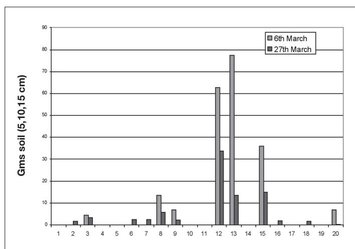
**Figure 3:** Relative soil loss (grams) collected using MWAC aeolian dust monitors at each of the monitored paddocks on two sampling dates (6 and 27 March). Losses are the sum of the three lower monitors averaged over the three replicates per paddock.
