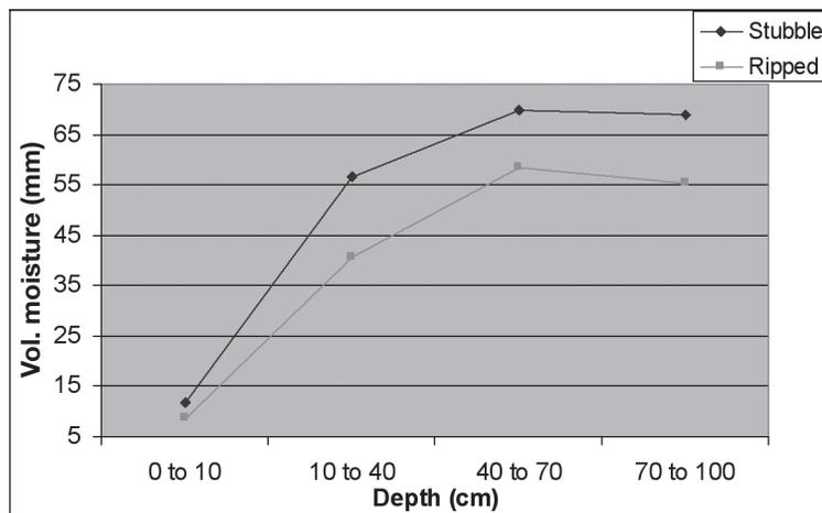
**Figure 2:** Volumetric soil moisture to a depth of 100cms from Wooroonock Sites 19 (Stubble) and 20 (Ripped) when sampled in January 2007.
