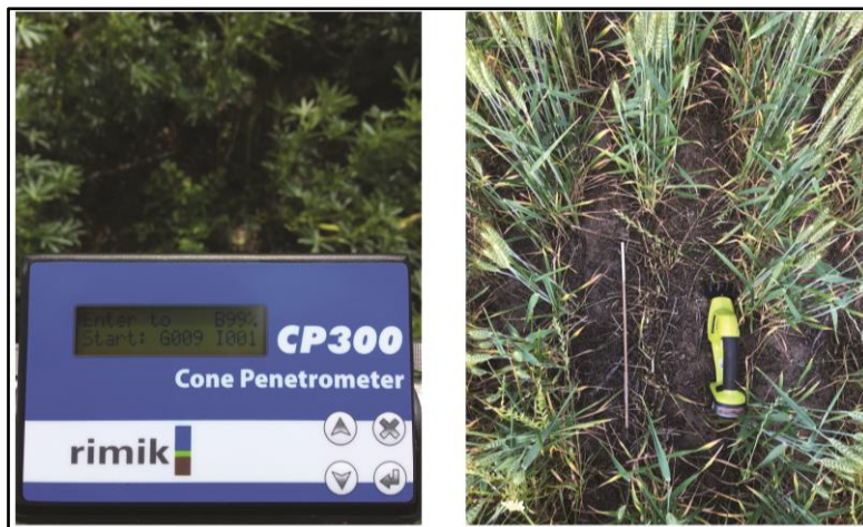
Figure 2: Cone penetrometer used to measure soil strength (left) and shears used to measure plant biomass (right)
