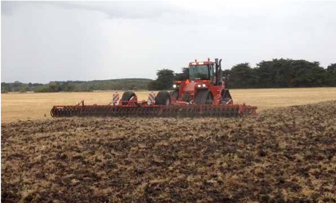
Figure 6. Horsch Speedtiller in action at Crop Walk in November 2014
