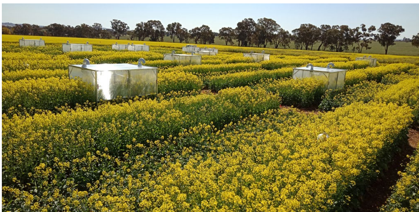
Figure 1 Heat chambers for assessing heat stress in canola plots at Wagga Wagga Agricultural Institute.
