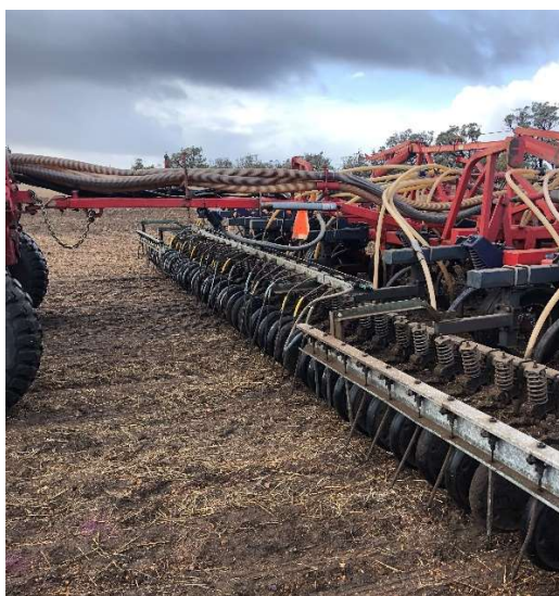
Figure 1: Photo of the liquid delivery system used to apply soil wetting agents by Michael Webster and his family. The wetter is applied directly onto the seeding furrow behind the press wheel. The photo was taken by Nathan Dovey- Stirlings to Coast Farmers on the 6th of May 2021.
