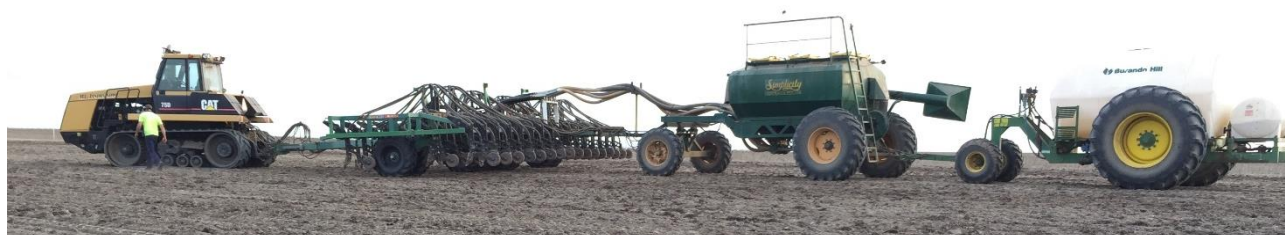
Photo 1. DBS seeding bar and liquid cart used to seed demonstration site on the 18 th May 2016.
