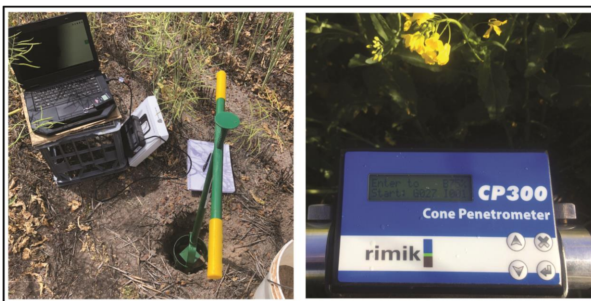
Figure 18: 3D scanning equipment used to calculate bulk density (left) and soil strength (right).
