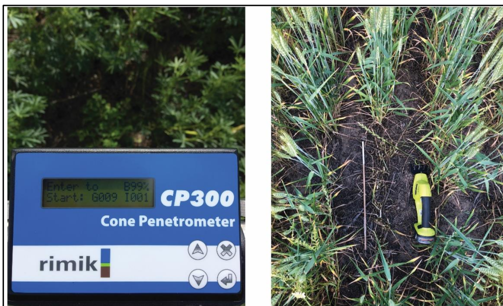
Figure 16: Cone penetrometer used to measure soil strength (left) and shears used to measure plant biomass (right)
