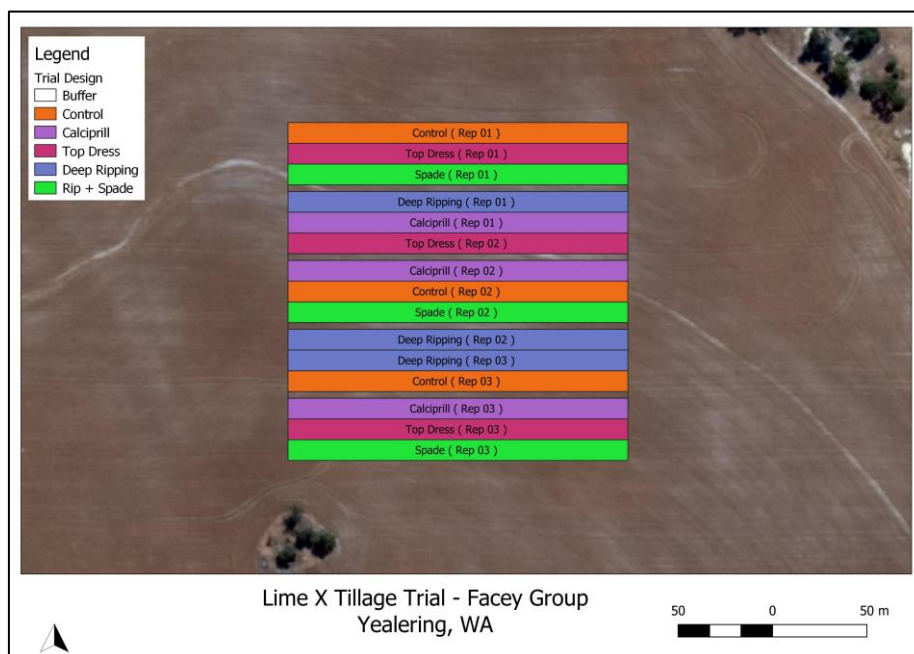
Figure 17: The Facey Group Inc lime and tillage trial was finalised in 2017. The trial consisted of two lime treatments and three ripping treatments in 11 metre wide plots. Undisturbed 'Control' plots allowed yield comparisons to be made in the 2018 canola crop.
