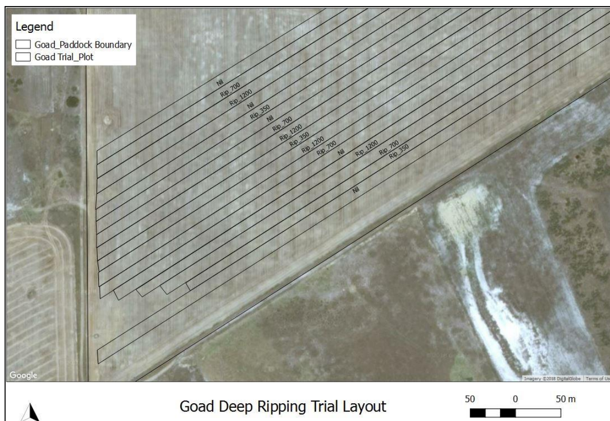
Figure 1: The deep ripping trial design on Josh and Tony Goad's farm near Kojaneerup was finalised in 2016. The trial consisted of three ripping treatments at 350mm, 700mm and 1200mm in 12 metre wide plots. Undisturbed 'Nil' plots allowed yield comparisons to be made in barley, canola and barley crops in 2016, 2017 and 2018.
