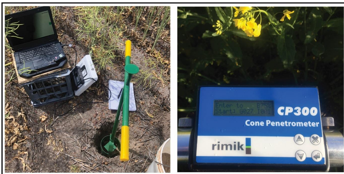
Figure 2: 3D scanning equipment used to calculate bulk density (left) and soil strength (right).
