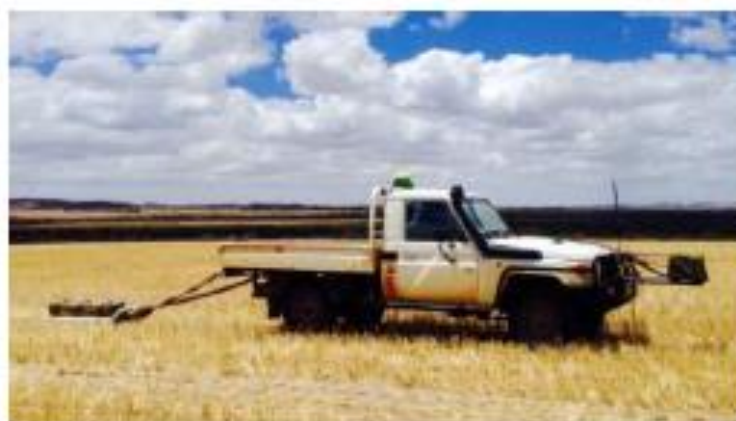
Photo: Electromagnetic and gamma radiometric being collected at Wickiepin for the GRDC RSCN Kwinana West Project. (Source: Kieran Brennan)
