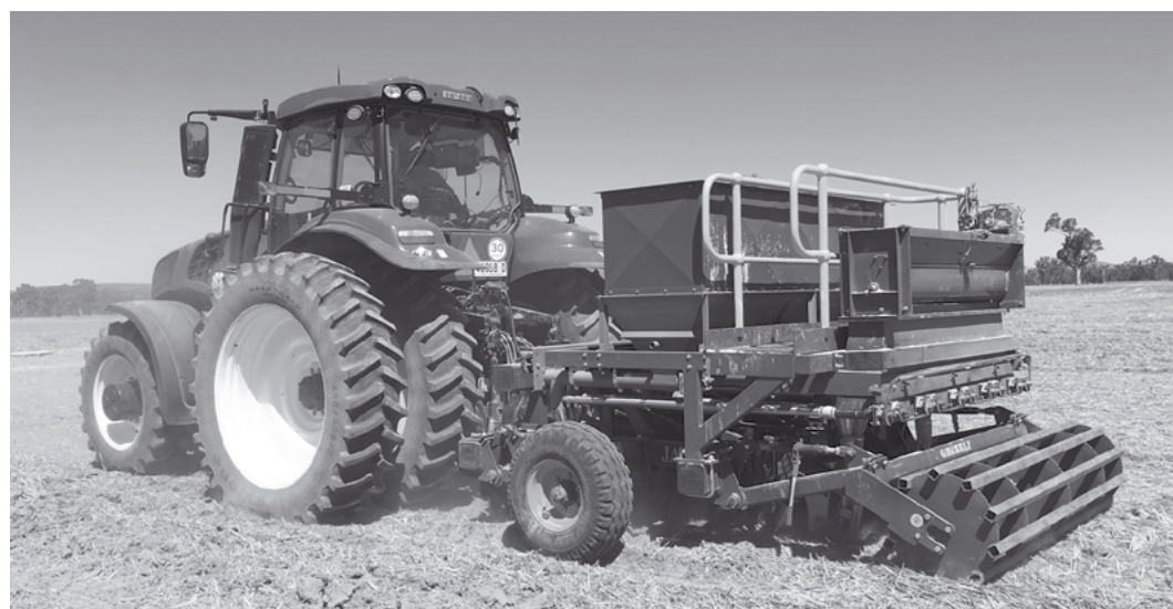
Figure 2. 3-D Ripper, designed and fabricated by the NSW Department of Primary Industries.
