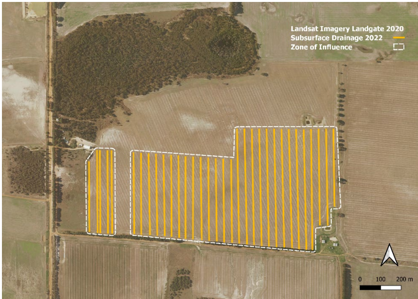
Figure 2: Dalyup sub-surface drainage trial in the Esperance Port Zone (Source: South Coast NRM 2024b).
