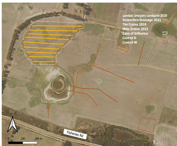
Figure 4. Neridup Subsurface Drainage Trial Design.
