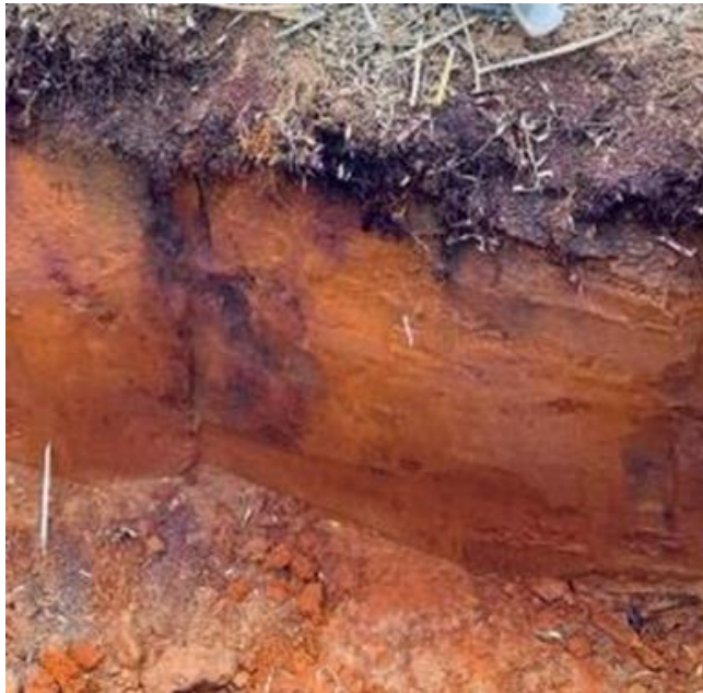
Photo 1. Soil pit face of a plot deep ripped with inclusion plates to incorporate lime. Acid test indicator has been sprayed on the surface and purple colours show the level of lime incorporation. The yellow and red colours show slightly acidic to acidic soil that has not been affected by the application of lime. Photo taken April 2022.
