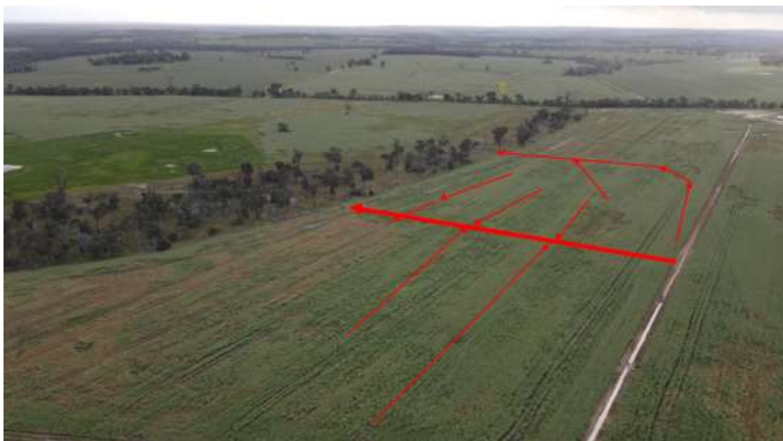
Figure 4: Drone imagery capturing waterlogging conditions experienced on 5th October 2022 and a visible reduction in plant health evidenced in the control region to the left of the drainage lines. (Source: Stirlings to Coast Farmers Inc.)
