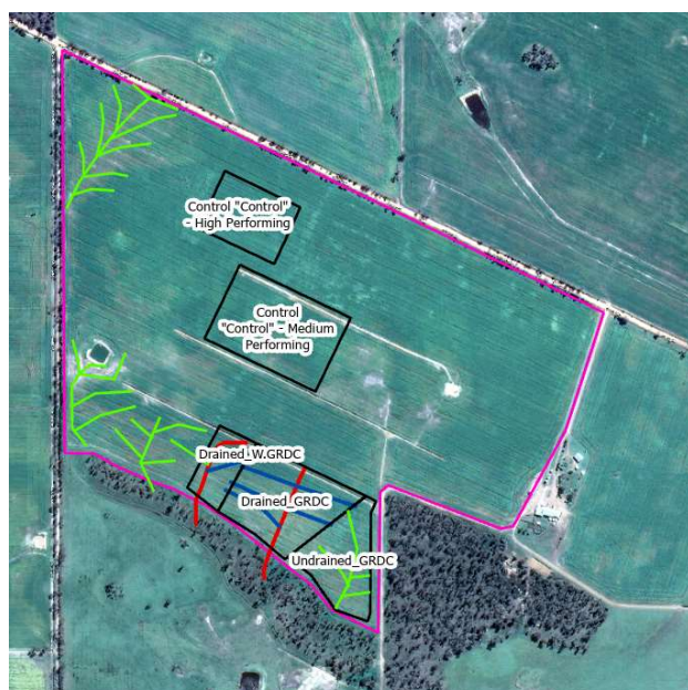
Figure 10: Hypothesised potential sub-surface drainage layout to be utilised in a simplistic ROI calculation
