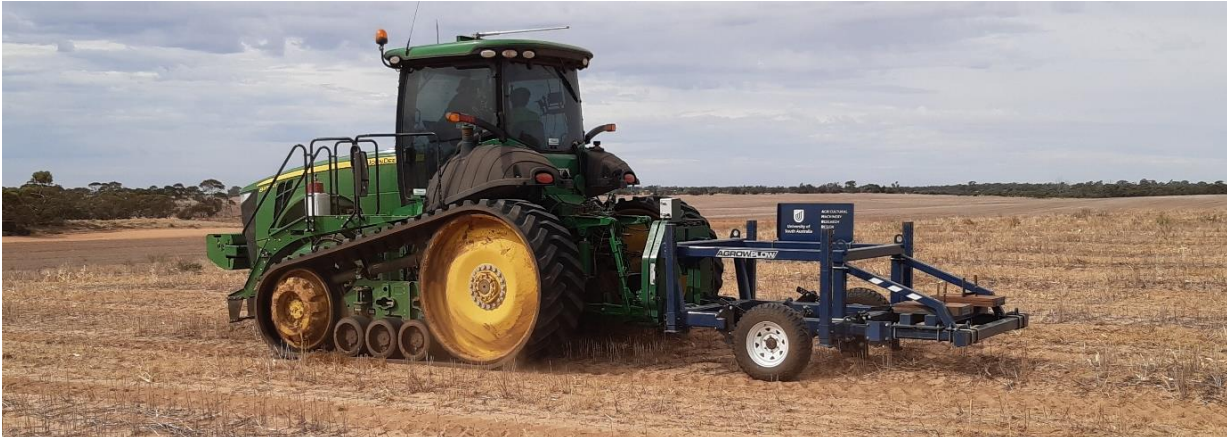
Image 1: Research conducted over the last 2 years in Mallee sandy soils used a research ripper frame with draft force measuring capability to quantify the impacts of a selection of deep ripping tyne designs on soil loosening efficiencies (Image: University of South Australia)
