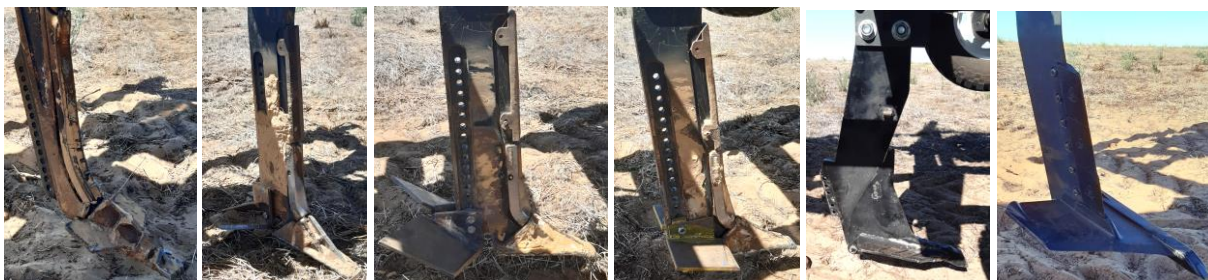
Image 4: Narrow shank ripper tynes with wings evaluated in Mallee trials (Images: University of South Australia) L to R: Agrowplow #9 shank with 210mm winged blade (35mm lift); Tilco Ag Systems rigid shank with i) 290mm wide Delta wings (20mm lift); ii) with UniSA 310mm wide square wings (40mm lift); iii) with UniSA 310mm wide delta wings (95mm lift); He-Va Subtiller shank with 200 mm wide wings (50mm lift) and Agrisem Cultiplow TC750 shank with 320mm wide wings (80mm lift) and 160mm offset 47mm wide point.
