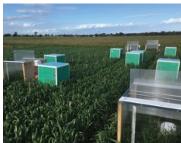
FIGURE 2 Simulated frost chambers in the field experiment, Horsham, Victoria, 2016
