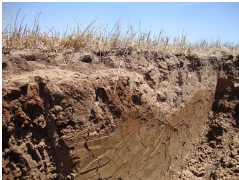
Figure 1. Distinct soils in the high rainfall zone consist of light surface soil over a dense clay subsoil.
