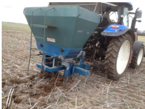
Figure 2. Placing chicken manure to a depth of 40cm using the SFS 2 leg subsoiling machine with hopper
