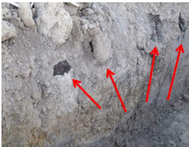
Figure 3. Arrows indicating manure placed at depth by the subsoil machine
