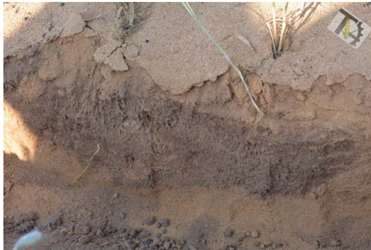
Photo 5: Mouldboard burying of lime and topsoil below toxic subsoil.
