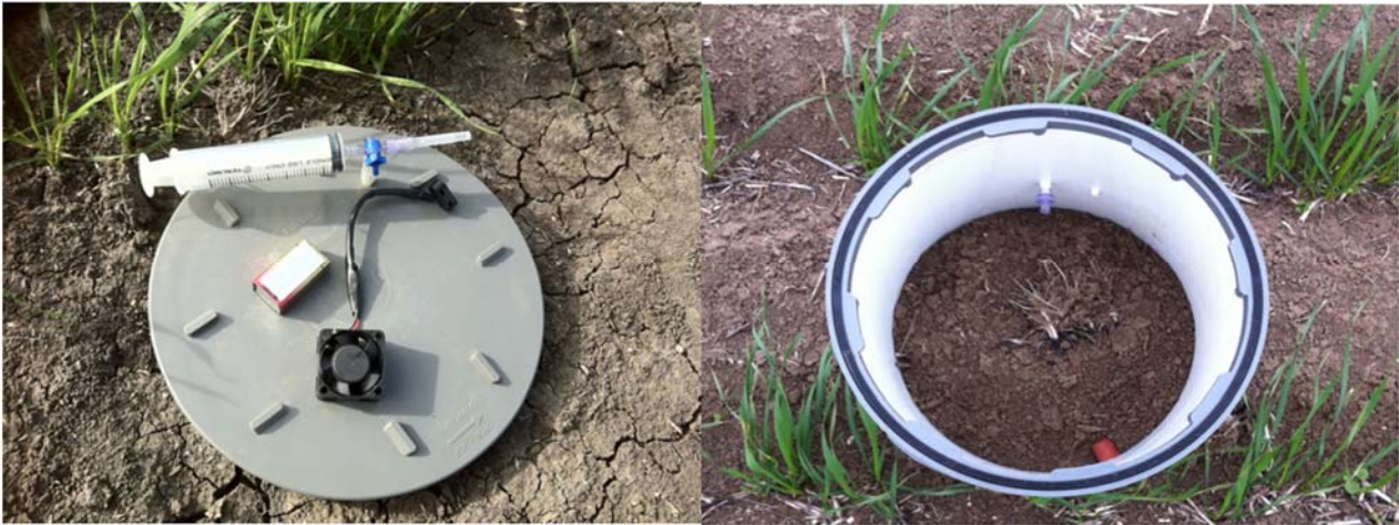
Figure 2: N 2 O sampling cylinder (right) with lid and syringe to extract samples from the cylinder (left)
