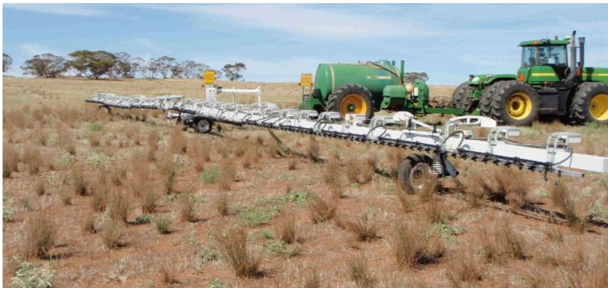
Figure 2. Optical sensing technology such as the WEEDit™ system can dramatically reduce summer spraying costs and help control "hard to kill" summer weeds by using higher doses of herbicide and/or more expensive products. Photo: Ed Cay
