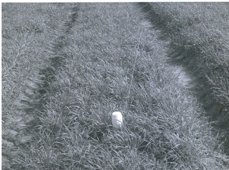
Photo 11: Tube installed for neutron probe assessment of soil moisture
