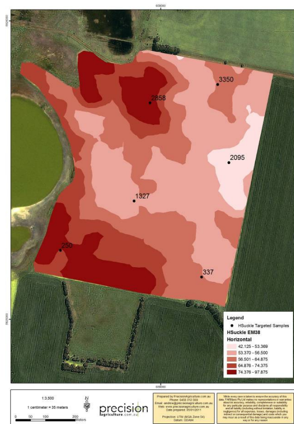
Image 1: EM38 (horizontal) map with locations of strategic soil samples
