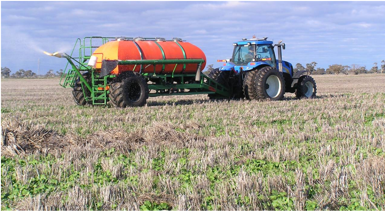
Ausplow DBS bin with whale tale with Topcon X20 controller, Autofarm RTK steering.
