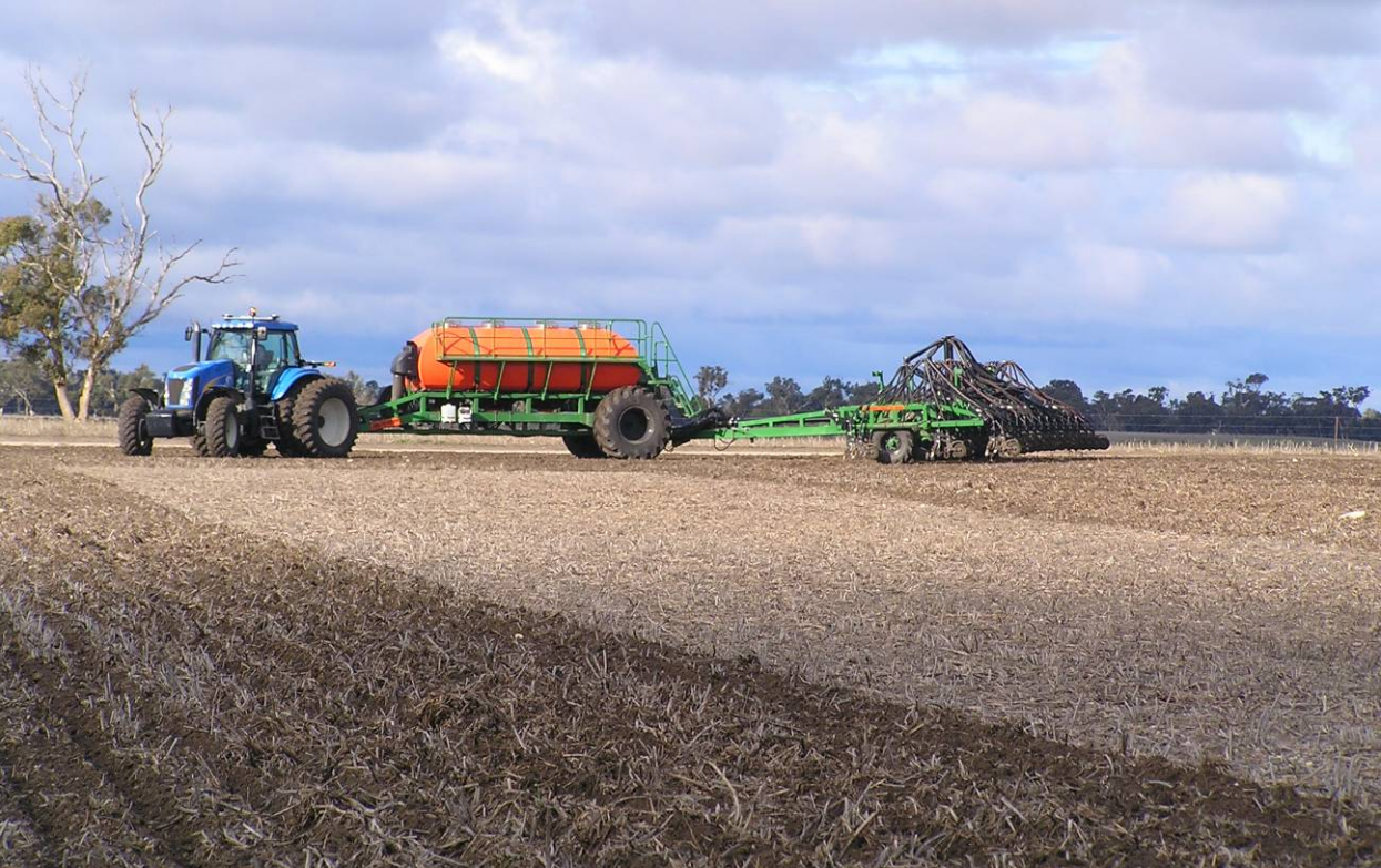
Ausplow DBS airseeder with Topcon X20 controller and Autofarm A5 RTK steering.
