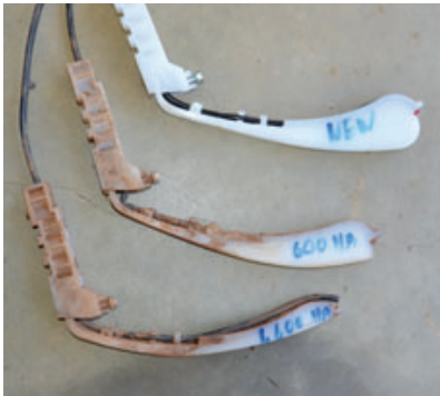
FIGURE 4: THE SEED FIRMERS HAD A HIGHER WEAR RATE AND WERE LESS DURABLE THAN THE LOCK-WHEELS ON EACH OF THE FARMS WHERE THE SIDE-BY-SIDE EVALUATION WAS CONDUCTED. WEAR IS SHOWN AFTER 600HA AND 1,600HA.
