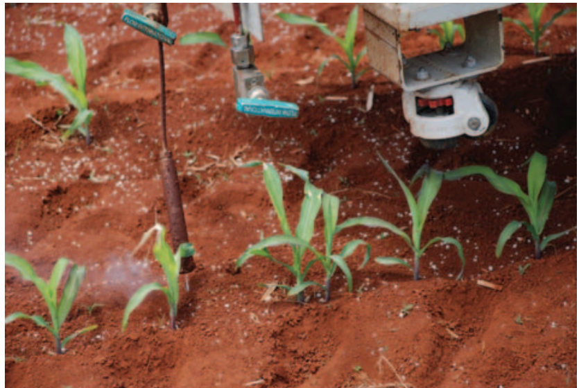
THE UHP JET, WHICH DID A GOOD JOB OF UAN INJECTION, CAN ALSO CUT THROUGH HEAVY SURFACE RESIDUE, THOUGH THAT WASN'T NEEDED IN THIS NSW CORN CROP.
