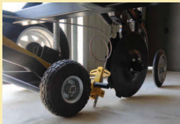
FIGURE 3: THE AQUA-TILL ULTRA-HIGH-PRESSURE LIQUID CUTTING NOZZLE FITTED TO A PARALLELOGRAM SYSTEM IS TO BE TESTED AS A LIQUID COULTER IN 2015.
