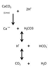
**Reaction 1.** In wet and acid soil, calcium carbonate in lime (CaCO3) breaks up into calcium and carbonic acid (H2CO3). This reaction can be rapid under acid conditions or extremely slow if pH(Ca) is greater than 5.8 (Whitten, 2000).
