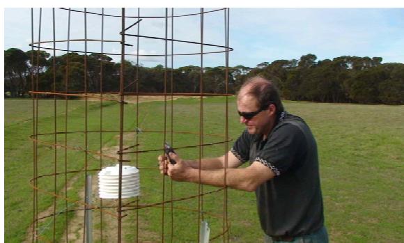
IMAGE 2 Geoff Nutt (KI farmer) assembles logger screens inside protective mesh cages
