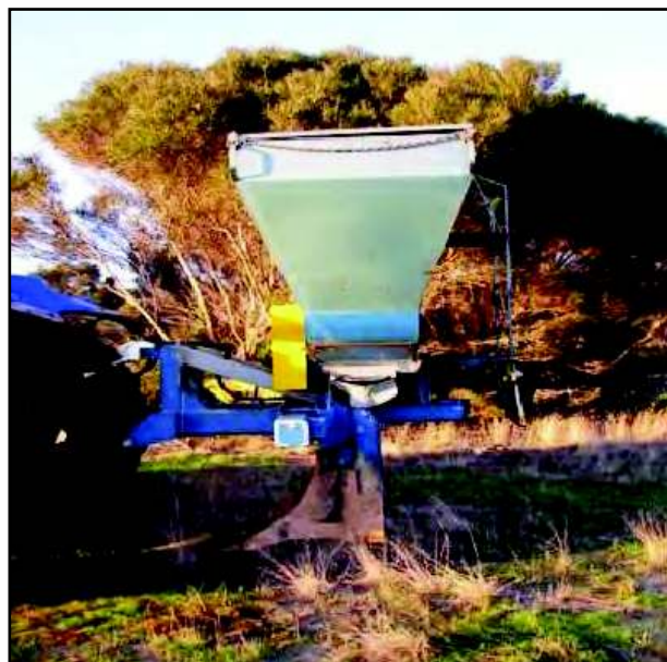
Sub soiler machine
