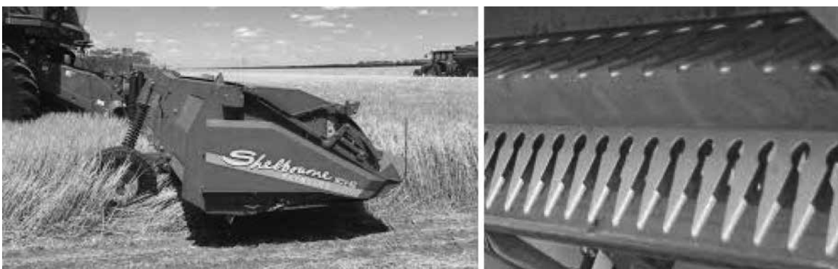
Figure 1. A Shelbourne stripper front designed to harvest grain heads and leave maximum crop residue.
